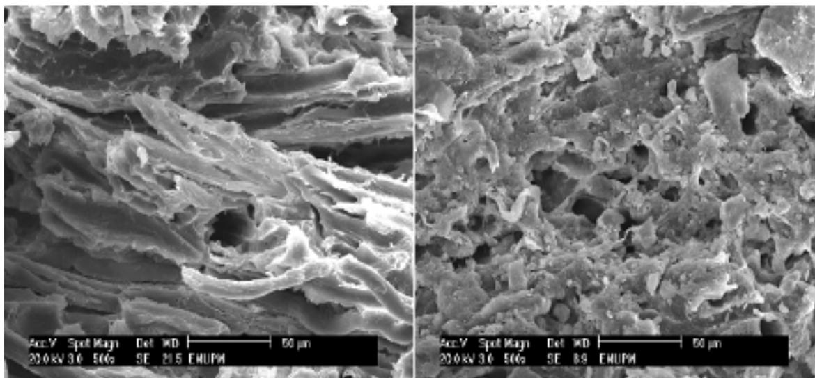
**Figure 4.** Scanning electron micrographs (Mag.  $\times 500$ ) of the fracture surface of 50%cellulose+5%PEG for LDPE (Left) and 50%cellulose+7%PEG for HDPE (Right) composites after 4 months in the soil
